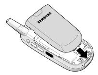
**5.** Press the battery down until it clicks into place. Make sure that the battery is properly installed before switching on the power.
